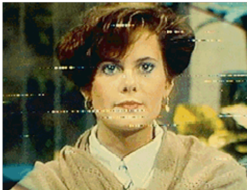
Picture 7: Electrical Interference -- low noise
